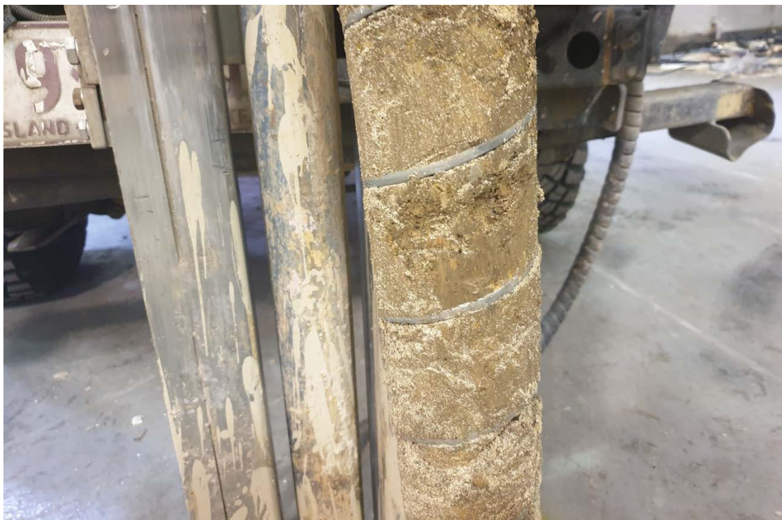
Photograph 6: Image of natural clay materials sampled from auger drill, encountered within BH107 (25 October 2019).
