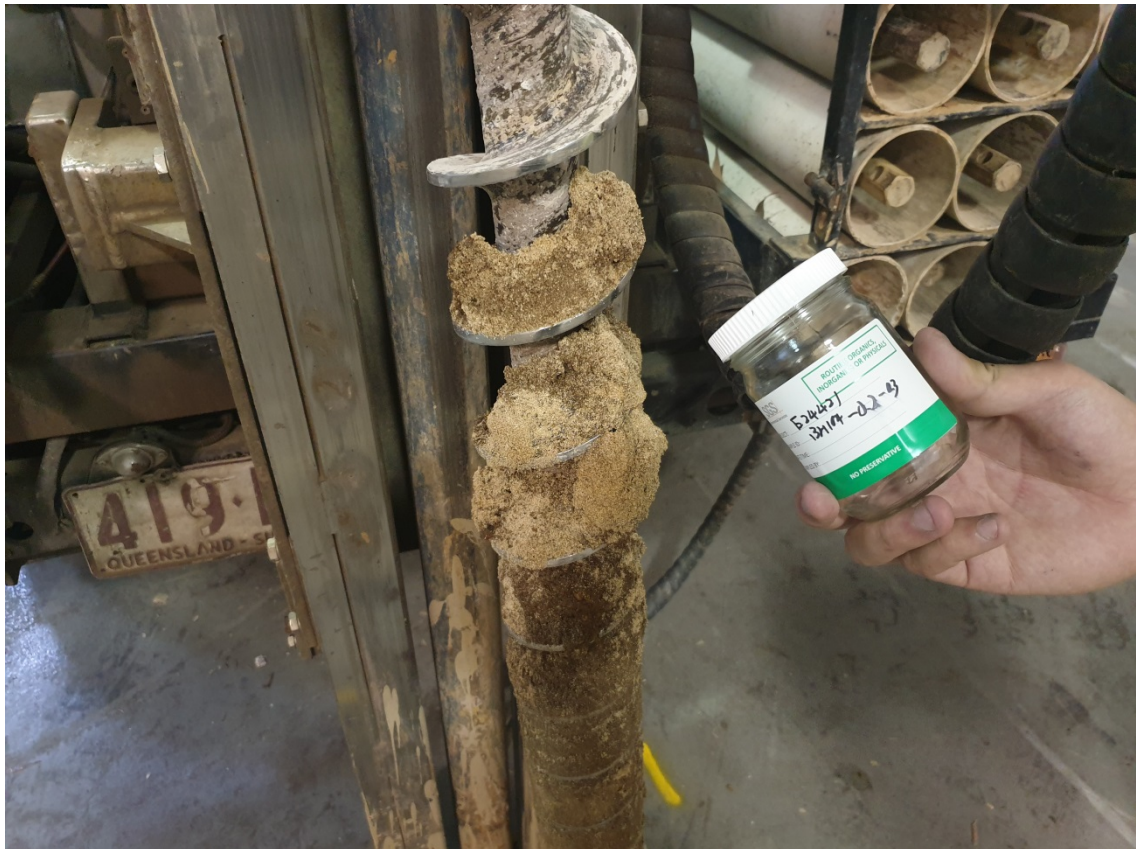
Photograph 5: Image of fill materials sampled from auger drill, encountered within BH107 (25 October 2019).
